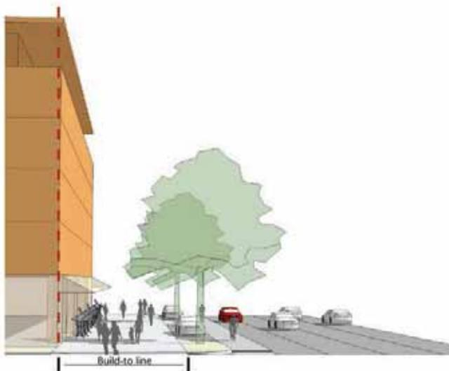
Figure 7.4 | Illustration of Pedestrian Space Measured from Building Face to Start of Sidewalk
